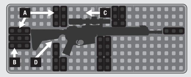
DAKA® GRID Blocks are engineered to absorb high impact forces and provide superior impact protection over open cell sheet foam. DAKA GRID Blocks are designed to be a sacrificial point of failure — this protects your gear and reduces chance of case damage. If a heavy impact occurs, inspect contents and blocks, and reorient or replace blocks as needed.
