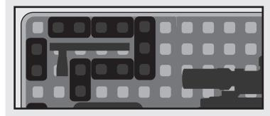
Remove a center GRID Panel: If the accessory is still too wide, a center panel can be removed to create more space without degrading the overall support of the system.
