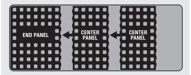
Once all CENTER panels are in case, place END panel against right hand edge and angle both the last CENTER panel and END panel upwards so they form a tent.
