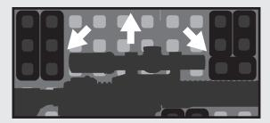
Fitment against equipment will not always be exact — Once lid of case is closed, top foam will compress GRID and secure stowed items.
