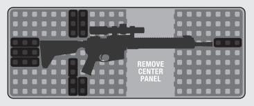
Cutting a GRID Panel: As a last resort, you can cut a relief in base panel to allow large accessory. Ensure that the opening is large enough to accommodate the attachment and the firearm is securely braced in the GRID panel system.
